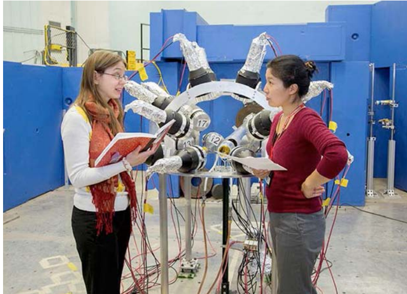
D. Neudecker and H. Y. Lee discuss the ^{235}\text{U} data in the Chi-Nu experimental area. Behind them is an array of neutron detectors surrounding the fission chamber.
