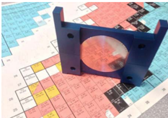
Scandium target before (left) and in a hot cell after irradiation (right).
