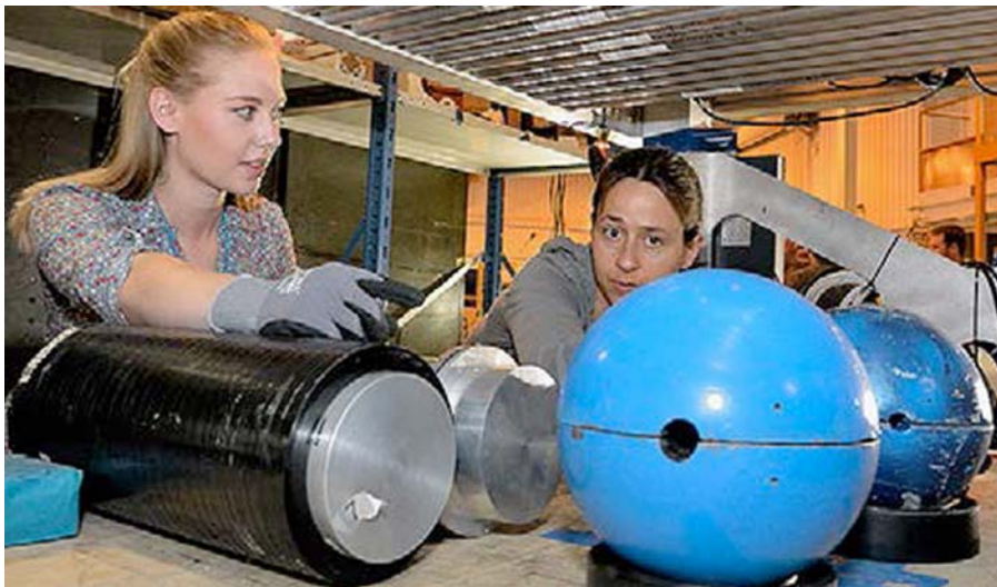
Los Alamos National Laboratory postdoctoral researcher E. Guardincerri (right), and undergraduate research assistant S. Fellows (left) prepare a lead hemisphere inside a muon tomography machine.
