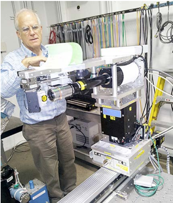
R. Sheffield checks distances for lens focal length and efficiency measurements at the APS 1-ID beamline.
