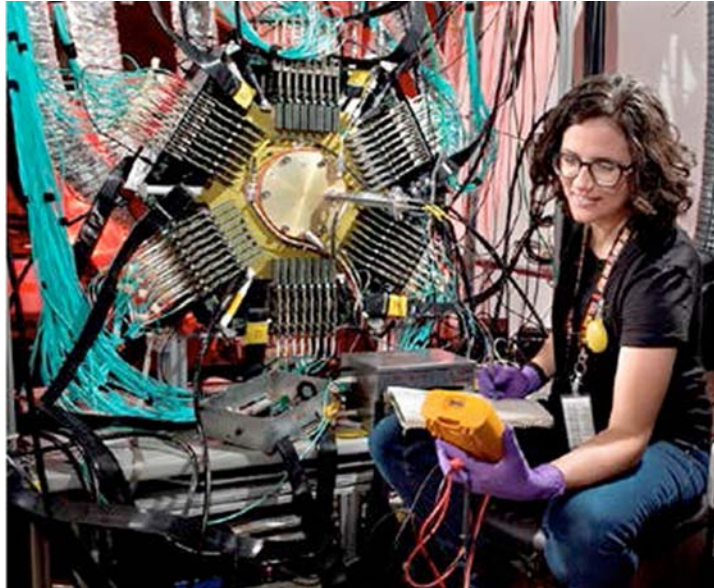
V. Kleinrath with the fission TPC, which she uses to perform this work as part of her PhD thesis at Vienna University of Technology.
