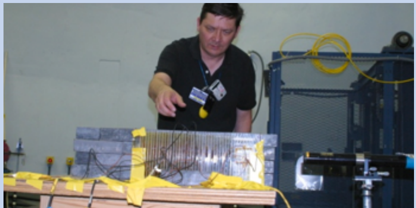
A University of New Mexico researcher assembles a stack of semiconductor devices for testing in the Weapons Neutron Research facility's proton beam.
