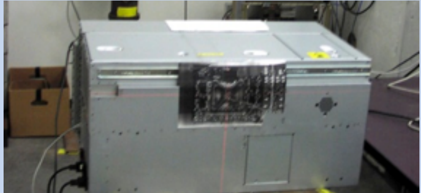
One module of Los Alamos National Laboratory's Q-Machine supercomputer being tested in the Weapons Neutron Research facility's neutron beam.
