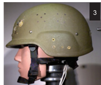
Figure 1) Proton radiograph of a jet penetration (penetration direction bottom to top). Figure 2) Optical photograph of an armor material cross section acquired after impact of a kinetic energy projectile (impact direction top to bottom). Figure 3) Optical photograph of a composite material helmet just prior to a kinetic energy projectile impact (projectile moving from right to left).
